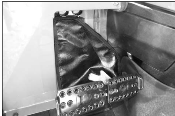
Fig. 13.1 (Vinyl Filler installation)
