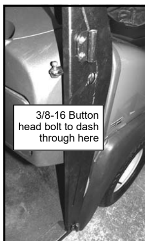
Fig. 2.2: Frame to Dash bolts
