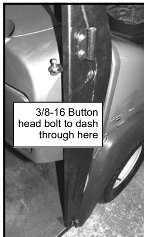
Fig. 2.2: Frame to Dash bolts
