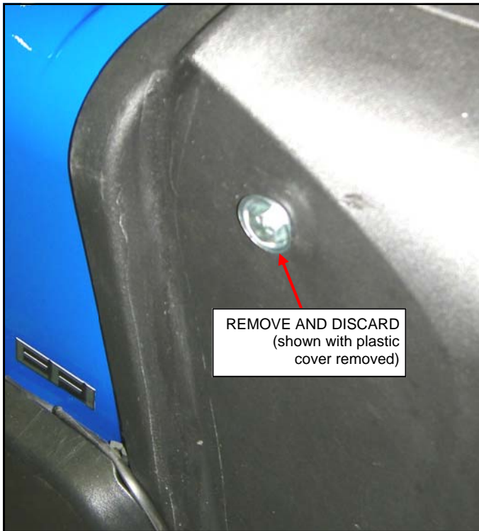
Figure 1.2: Dashboard Side Bolts
