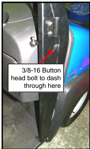
Fig. 2.2: Frame to Dash bolts
