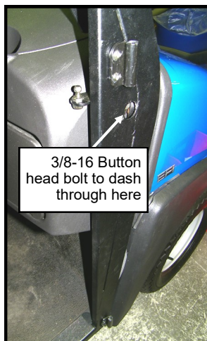
Fig. 2.2: Frame to Dash bolts
