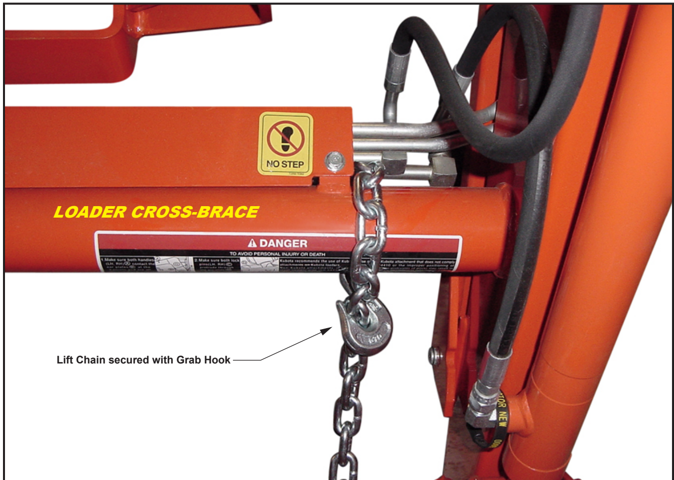
Figure 13. Loader Blade secured with Lift Chain
