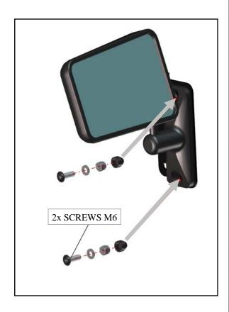
Remove screws and washers from the door where shown. Place the mirror assembly onto the door panel. Attach using the same original hardware into the factory installed threaded inserts. **Note:** the bracket can mount to the door two ways. One way the mirror is more upward and forward, the other way the mirror is more downward and rearward. Downward and rearward tends to be more favorable for best viewing. Orient at the installer's discretion.
