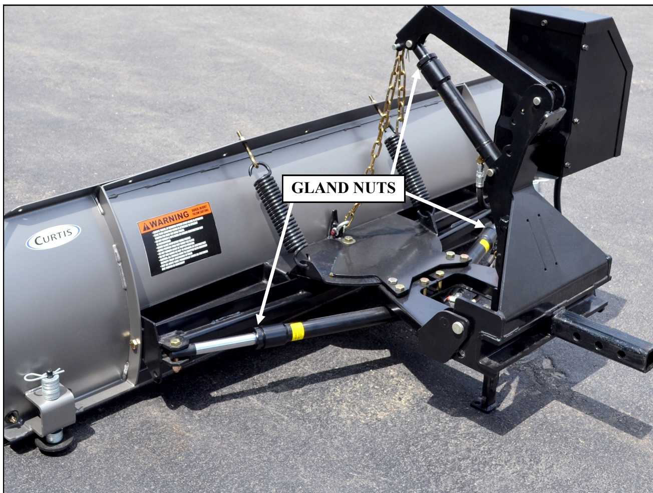
Fig. 11.3 repairing a Hydraulic Cylinder leak
