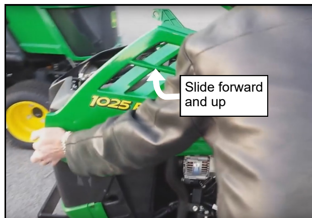
Fig. 3 (Slide forward and up)
