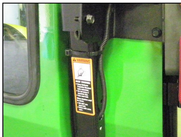
Fig. 26.1 (Avoid Crushing Decal on right ROPS Tube)
