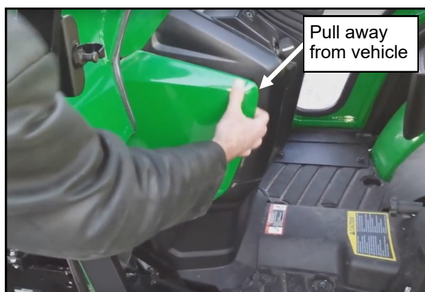
Fig. 2 (Pull panel away to clear slots)
