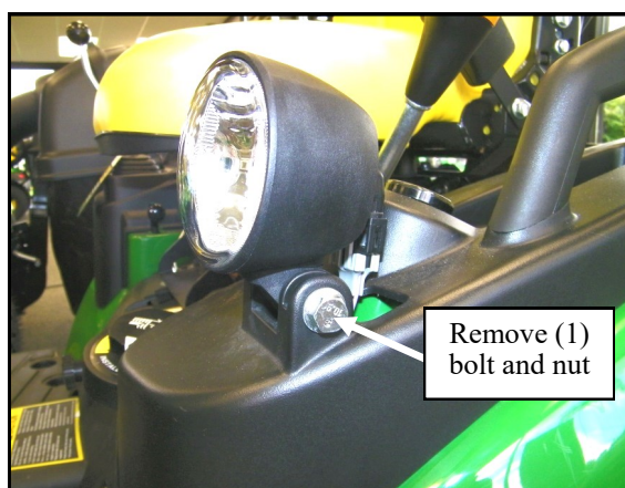
Fig. 1.1f (Fender Lights - Both Sides of Vehicle)
