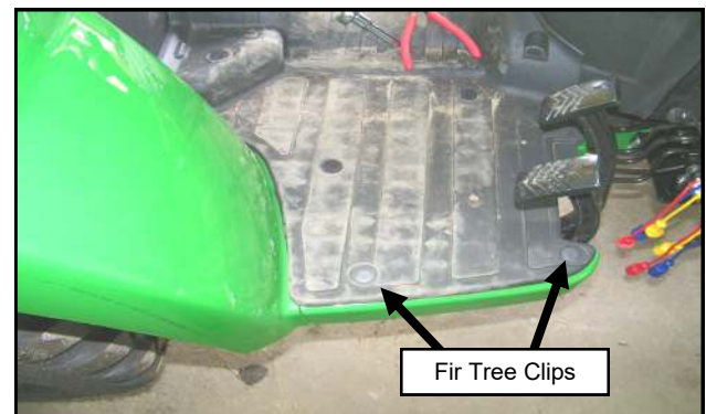
Fig. 1.3 (Remove Fir Tree Clips)
