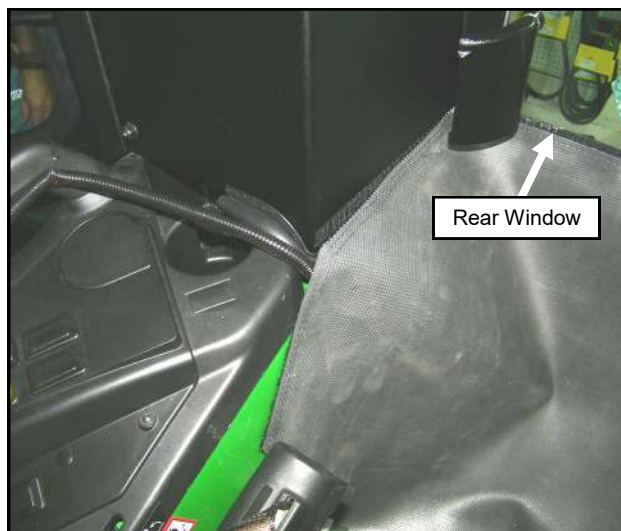
Fig. 19.2b (Install Under Seat Filler)
