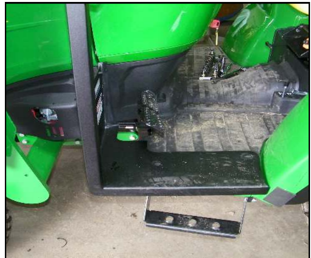
Fig. 5.1 (Loosely attach the left A-Pillar)
