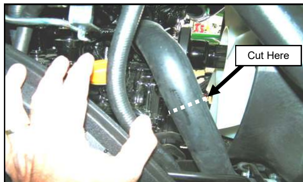
Fig. 17.2 (Cut Lower Radiator Hose)
