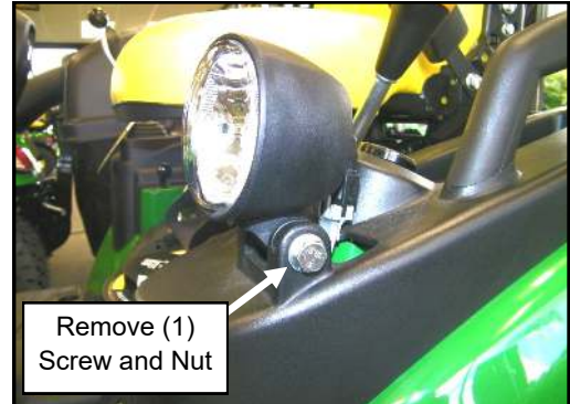
Fig. 1.1 (Remove Fender Lights)
