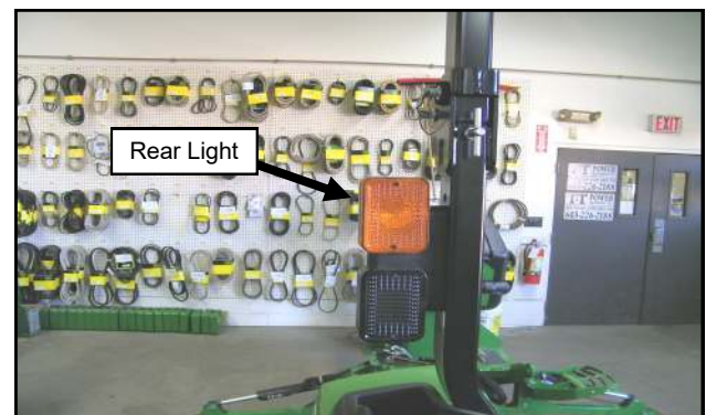
Fig. 1.2 (Unbolt Rear Lights)
