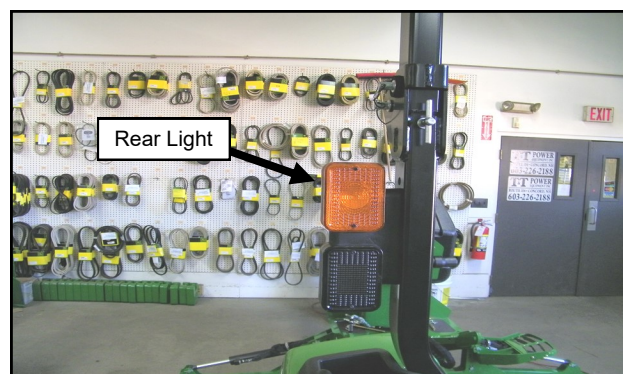
Fig. 1.2 (Unbolt Rear Lights)
