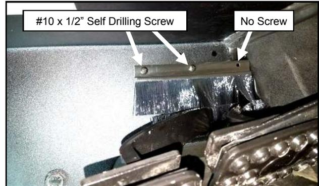
Fig. 2.1 (Attach Front Brush)
