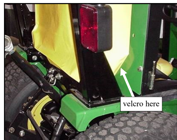
Fig. 13.4.1 Soft Side Curtain (viewed from the back)
