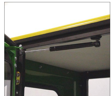
Fig. 10.2 Gas spring installation for hard sided doors only
