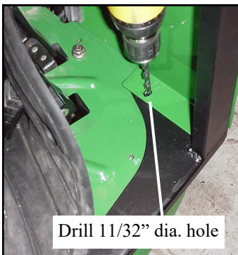
Fig. 9.1 Drill out Floorboard
