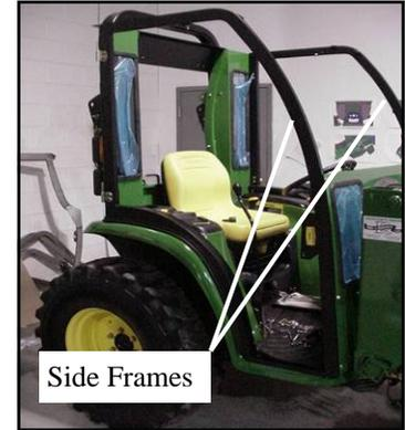
Fig. 4.2 Install Side Frames
