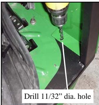
Fig. 9.1 Drill out Floorboard
