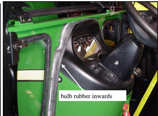
Fig. 3.3 front cowl installed (20 series shown)
