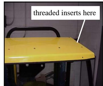
Fig. 7.1 Install Roof
