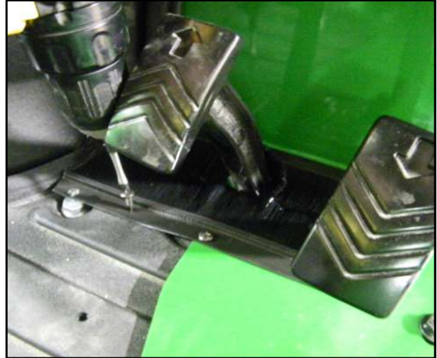
Fig. 2.1 (Attach Brushes to Right Floorboard)
