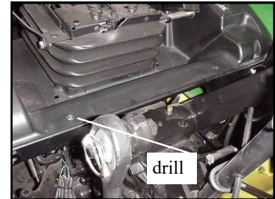
Fig. 1.5 Drill holes in plastic
