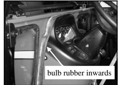
Fig. 3.4 front cowl installed (20 series shown)
