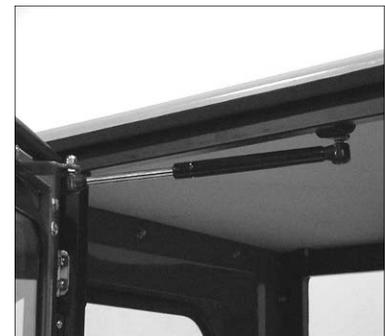
Fig. 10.2 Gas spring installation
