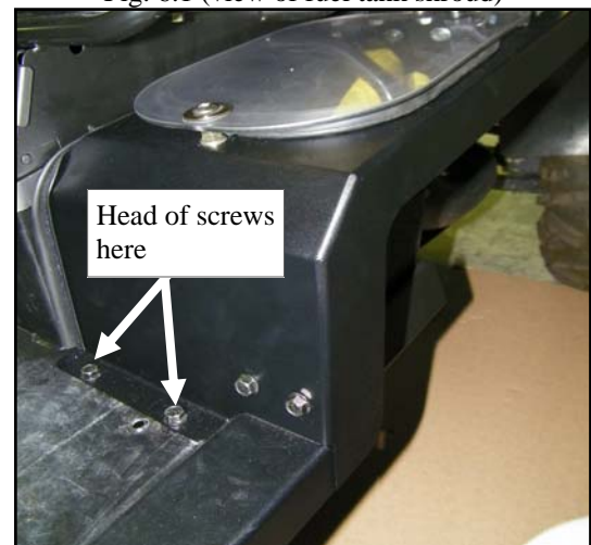
Fig. 6.2 (view of fuel tank shroud)
