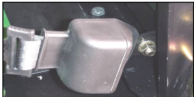
Fig. 20.2 (seat belt retractors)
