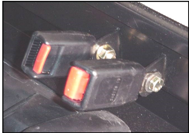
Fig. 20.1 (seat belt receivers )
