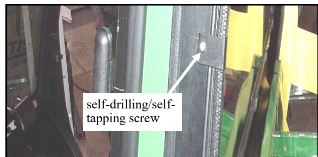
Fig. 18.3 (metal window clips) (view from driver's side)
