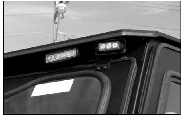
Figure 3b - Front Lights + Corner Flasher
