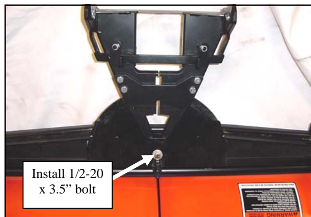
Fig. 7.2—Install A-Frame into Trip Frame Pocket
