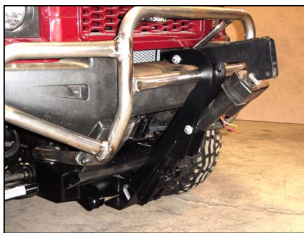
Fig. 2.3.1 — Lift arm mount assembly installation
