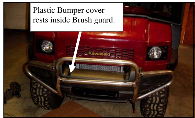
Fig. 1.5 — Brush guard installation.
