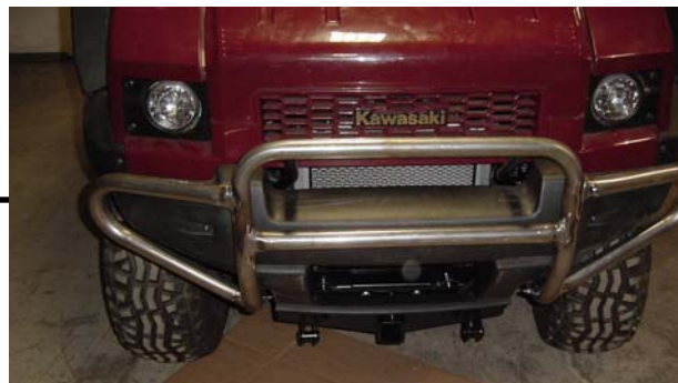
Fig. 1.8—Plow Mount Installed.
