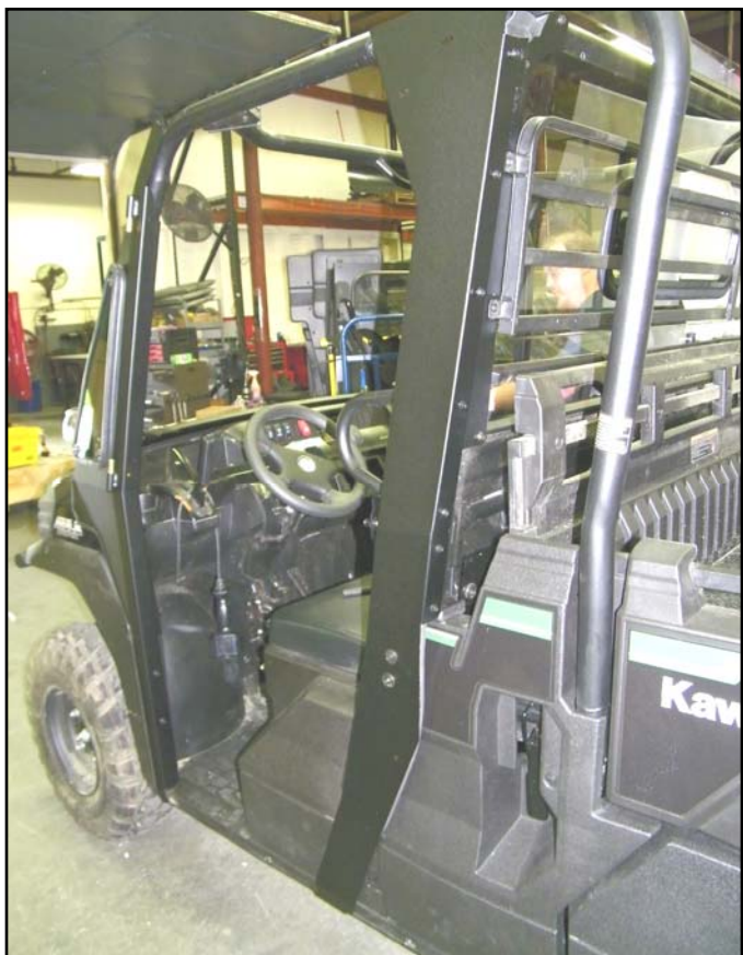
Fig. 3.3b B-Pillar, Driver Side
