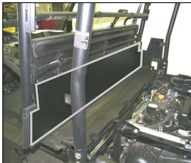
Fig. 2.2 Lower Rear Panel
