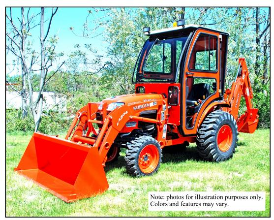
Hard sided cab shown with optional work lights, and optional strobe light. Additional options available are: heater, hard rear panel, and rear window wiper. Note: a front windshield wiper comes standard with this cab kit.
