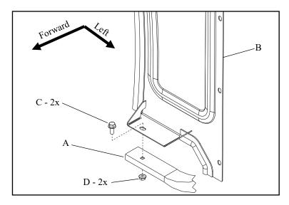
6. Install the left sideframe/door assembly making sure that the rear roll bar bracket is positioned on the inside of the ROPS as shown in step 7. (Note: Leave bolts finger tight)
