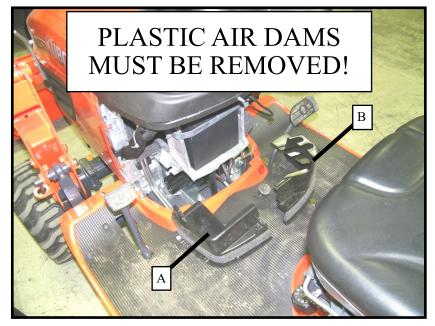
Note: For summer use the vinyl air intake panel should be removed to allow more air flow to the radiator.
