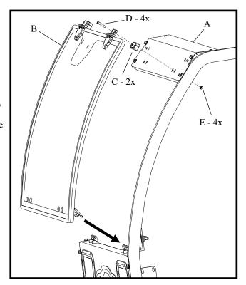
14. Place the roof in position on top of the cab. The latches may not engage properly and will be adjusted in a later step. Install the hinge pins as shown making sure the steel lip bolted to the rear of the roof is centered between the sideframes. To easily adjust the roof, loosen the bolts for the hinge sleeves that were factory installed on the roof and adjust in the mounting slots then tighten.
