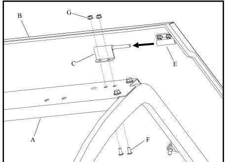
15. Open and close the roof to make sure that the steel lip at the back of the roof does not contact the sideframes. Once this is complete, attach the gas shocks to the ball studs with the thin rod end forwards. Loosen the latch bolts and adjust the latches forwards or backwards in the slots to obtain the best alignment with the pins on the sideframes.
