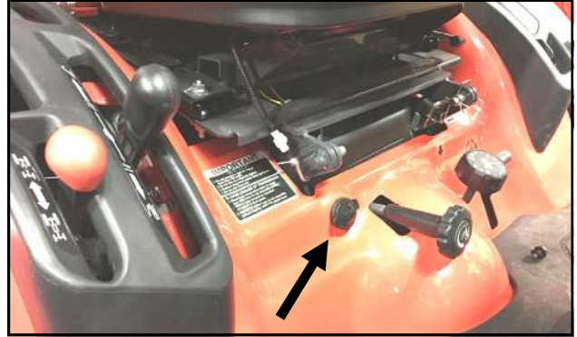
Fig. 2.10 (Remove Power Outlet)
