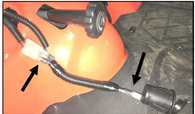
Fig. 2.11 (Connect Power Outlet to Wire Harness)
