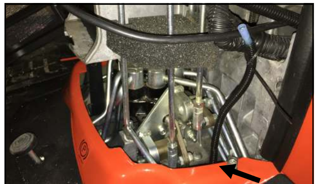
Fig. 2.13 (Wire Routing Into Battery Compartment)
