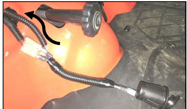
Fig. 2.12 (Wire Routing to Power Harness)
