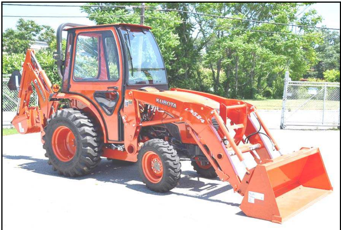
A hard sided cab is shown. A soft rear curtain is used when backhoe compatibility is required on a hard sided (all steel) cab.
