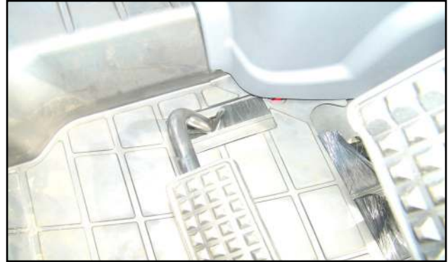
Figure 6.1 (Install a Drive Pedal Seal)
