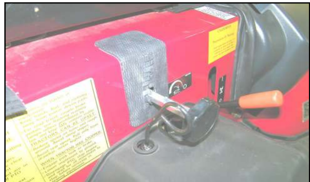
Figure 3.1 (Install Mower Knob Seal)
