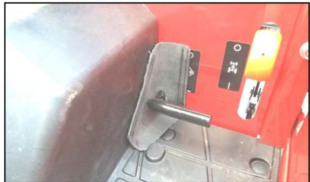
Figure 3.2 (Install Dif. Lock Seal)
