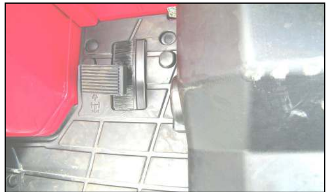
Figure 6.2 (Install Second Drive Pedal Seal)
