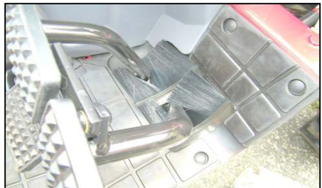
Figure 5.2 (Install Second Brake Pedal Seal)
