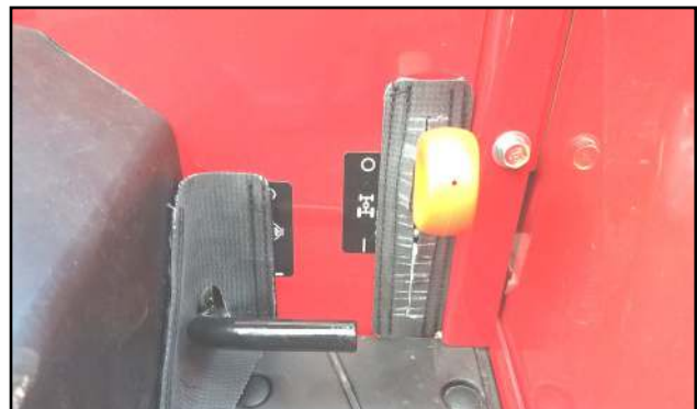
Figure 3.3 (Install 4x4 Lever Seal)
