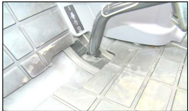
Figure 4.2 (Install Long Bristle Clutch Pedal Seal)
