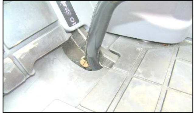
Figure 4.1 (Install Short Bristle Clutch Pedal Seal)
