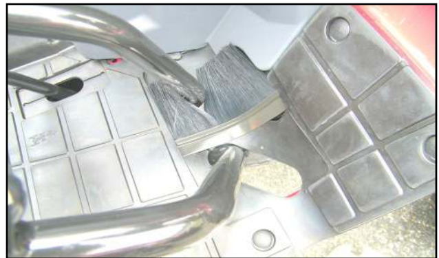
Figure 5.1 (Install a Brake Pedal Seal)
