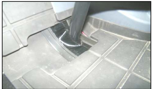
Figure 4.2 (Install Long Bristle Clutch Pedal Seal)
