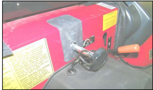
Figure 3.1 (Install Mower Knob Seal)
