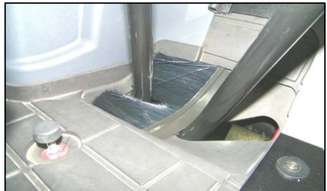
Figure 5.1 (Install Non-Chamfered Brake Pedal Seal)
