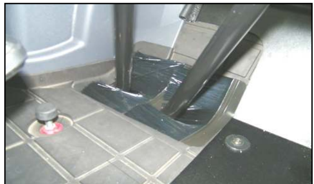
Figure 5.2 (Install Chamfered Brake Pedal Seal)
