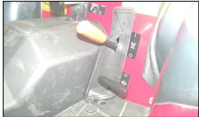
Figure 3.2 (Install Dif. & 4x4 Lever Lock Seal)
