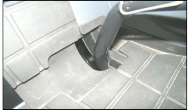
Figure 4.1 (Install Short Bristle Clutch Pedal Seal)
