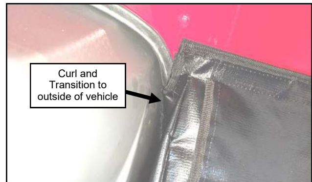
Fig. 1.5 (Transition Filler To Outside)
