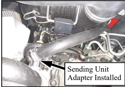
Fig. D-1 Adapter Installation
