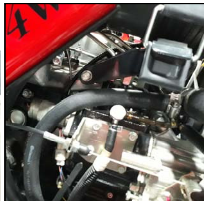
Fig. B-2 Heater Return Line
