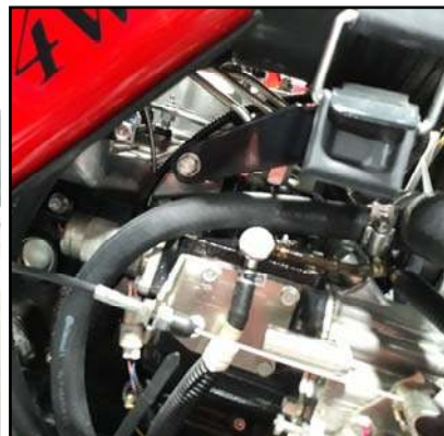
Fig. B-2 Heater Return Line
