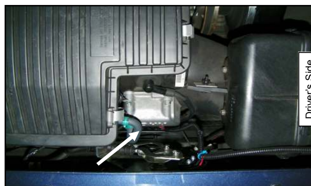
Fig. 4.9 (Connect to RPM signal wire)
