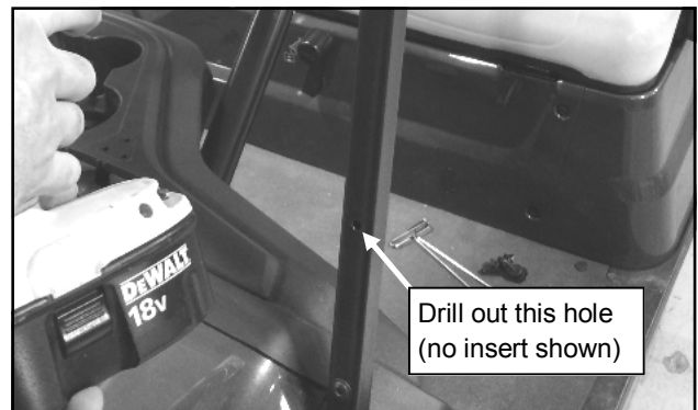
Fig. 2.5 (Drill Upper Hole)
