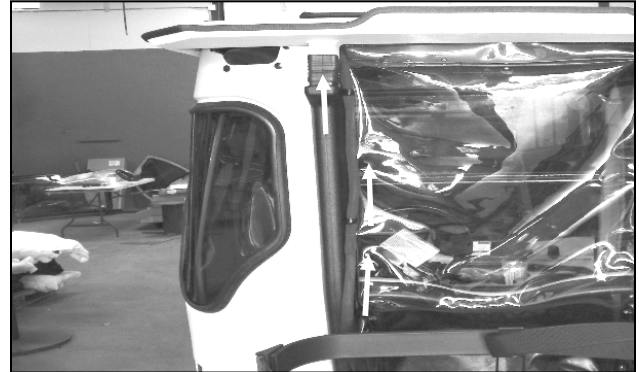
Fig. 5.1 (Route Wires to A/C)
