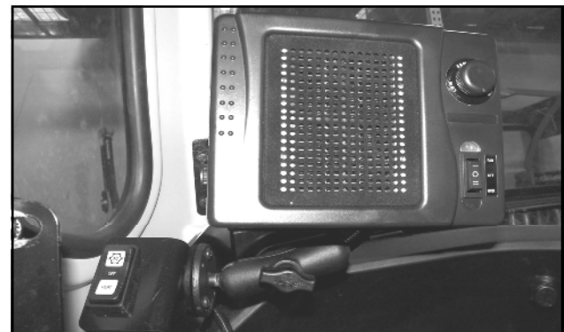
Fig. 2.11 (Install Heater and Clamp to Bracket)
