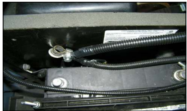
Fig. 1.4 (Disconnect Negative Battery Terminal)
