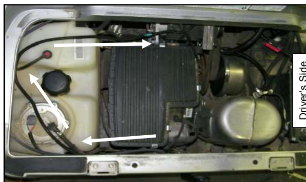
Fig. 4.10b (Route Signal Wire Harness 2016 & Older)
