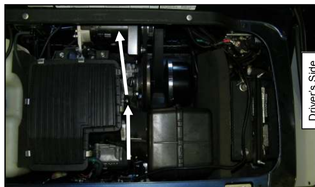
Fig. 4.10a (Route Signal Wire Harness 2017 & Newer)
