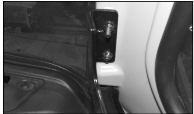
Fig. 2.10 (Install lower bracket hardware)
