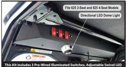
Dome Light, Plus a Circuit Breaker and Wiring for a Windshield Wiper
