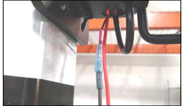
Fig. 10 (Black Wire to Light Connection)
