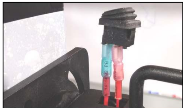
Fig. 9 (Red Wires to Switch)
