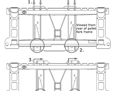
Once the Attachment is centered on the fork frame, **install the two Lock Keys** as shown on next page.
