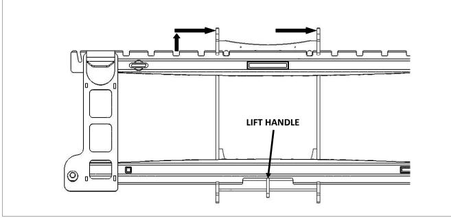
3. To install the outer Modules, <u>hang the upper hooks of the module in the fork rail detents</u> as shown below. The lower hooks should pass under the lower rail.
