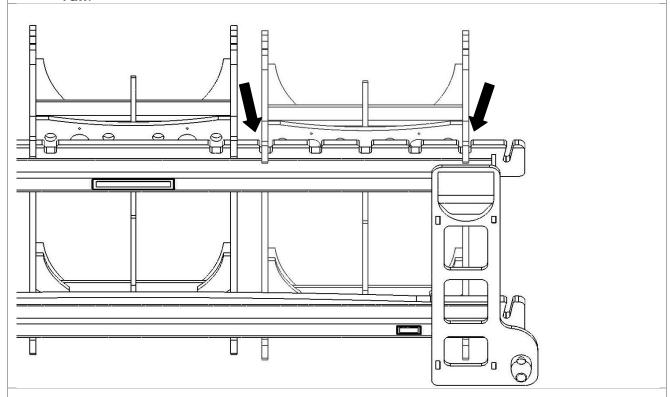
4. Using the Lift Handle, lift Module straight up and slide left or right, as desired.
