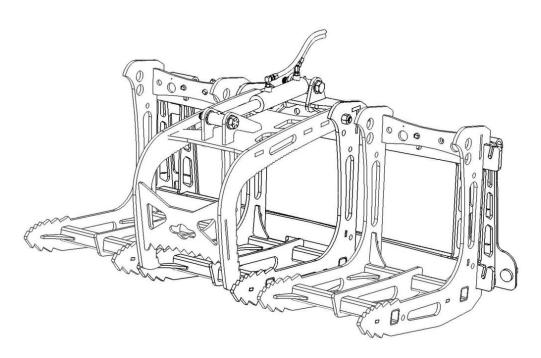
This is just one of several configurations of the Artillian Modular Grapple System. In this case, one Grapple Module is in the center with an adjacent Rake Module on each side. Many variations are readily achieveable and can be varied depending on the task at hand.
