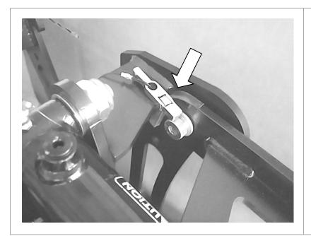
Grapple Module Lock Keys can be stored as shown.
