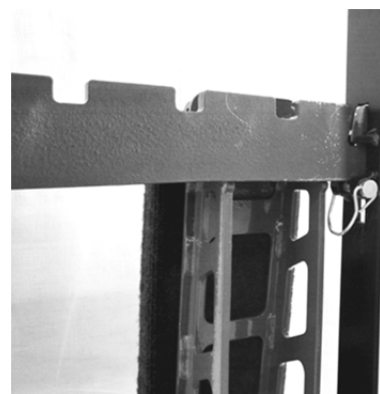
6. Latch Safety Wires on Pins (both ends)
