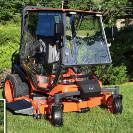
Kubota ZD1211 Featuring Optional Front Windshield Wiper, Side View Mirrors & Roof-Mounted LED Work Lights
