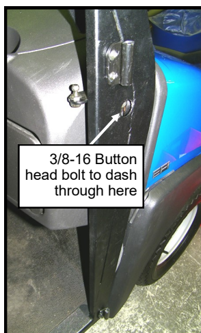
Fig. 2.2: Frame to Dash bolts
