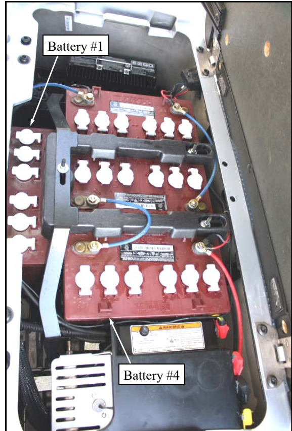
Figure 4.1 (view under passenger's side seat, four 12v battery configuration)
