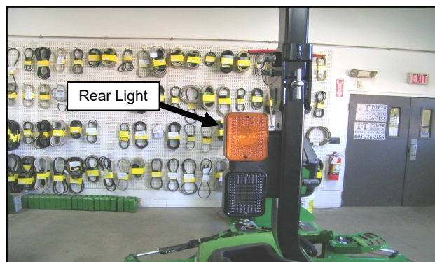
Fig. 1.2 (Unbolt Rear Lights)
