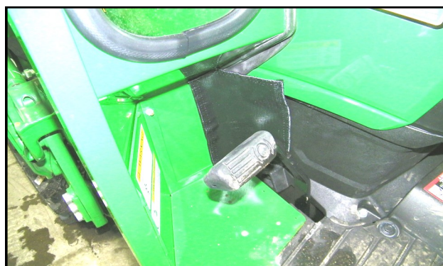
Fig. 25.2 (Install Front Filler)
