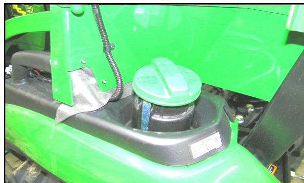
Fig. 6.1 (Wire Underneath Rear Leg)
