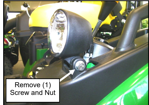
Fig. 1.2 (Remove Fender Lights)
