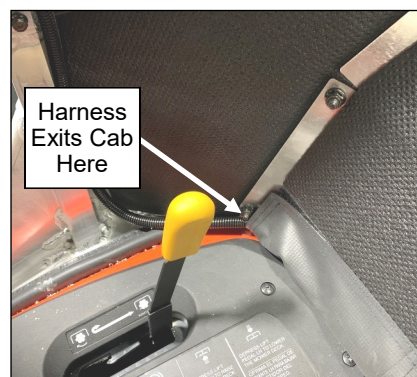
Fig. 1.20 (Run Wire out Under Rubber Filler)
