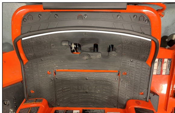
Fig. 4.6b (Seal location on 72")
