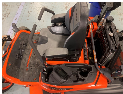
Fig. 5.1 (Move Seat forward, Rotate seatback)
