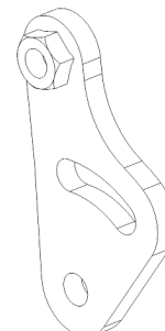
BRACKET, DYNAMO PIVOT P/N: 8SV-WA-00420
