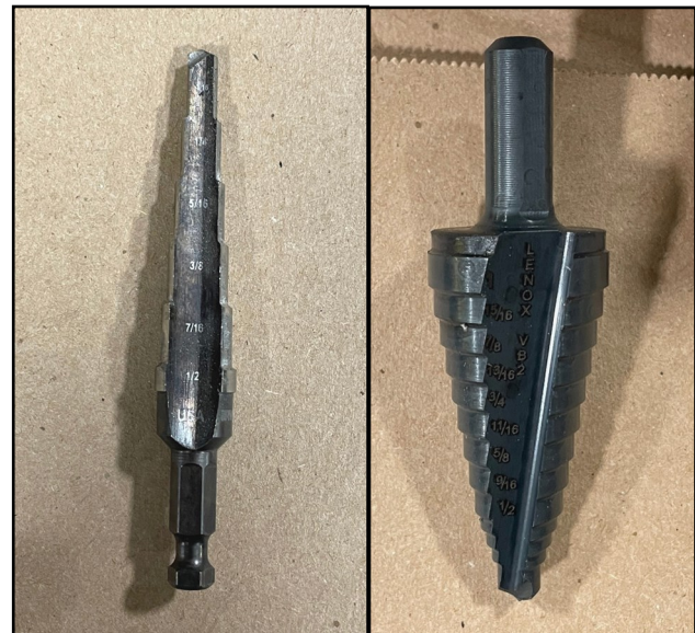
Fig. 1.7a (Recommended Step Drills)
