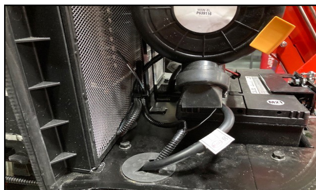
Fig. 13.9 (Coil Wires Behind Battery)
