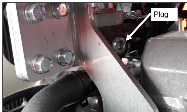
Fig. 14.2B (Remove Plug from Engine) CK3510, CK4010
