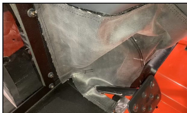
Fig. 17.2 (Install Front Filler)
