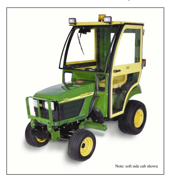
This Curtis Cab is designed and manufactured for use only as reasonable weather protection. This cab is not appli-cable, Nor should the cab be considered as protection against roll over, collision or other accidents that may result. This cab is NOT a R.O.P.S. cab. Extreme care should be taken when operating and by qualified, experienced operators only.
