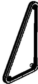
A-PILLAR WINDOW ASS'Y, RIGHT P/N: 8SV-9GL-00017-R
