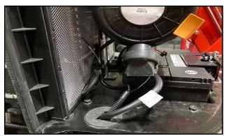
Fig. 13.9 (Coil Wires Behind Battery)
