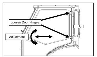
Fig. 18.3a (Door Hinge Adjustment)
