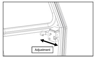
Fig. 18.3b (Door Latch Adjustment)
