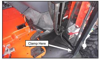
Fig. 13.4 (Wiring at Floorboard)
