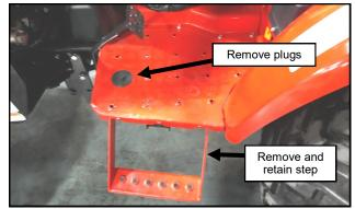
Fig. 1.4 (Tractor Floorboard)
