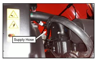
Fig. 14.5B (Supply Hose Routing)
