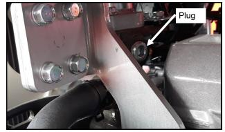
Fig. 14.2B (Remove Plug from Engine) CK3510, CK4010
