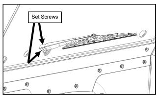
Fig. 15.3 (Wiper Arm and Blade)
