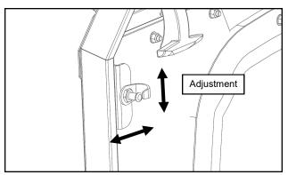
Fig. 18.4 (Striker Pin Adjustment)
