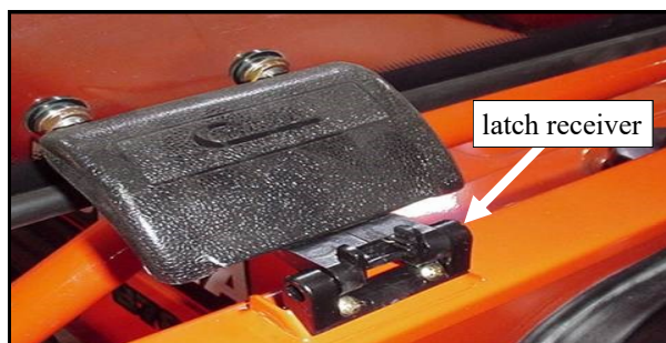
Fig. 9.2 (view from left rear side of tractor)
