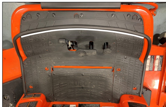
Fig. 4.6b (Seal location on 72")
