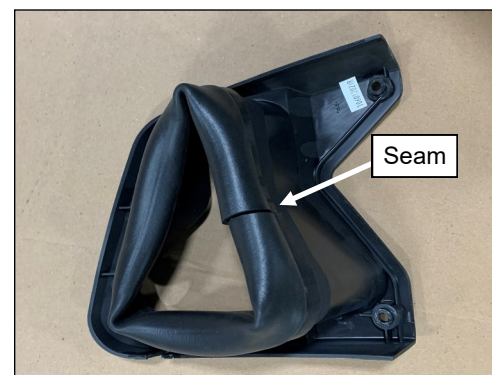
Fig. 1.5 (Install Rubber (Left shown))
