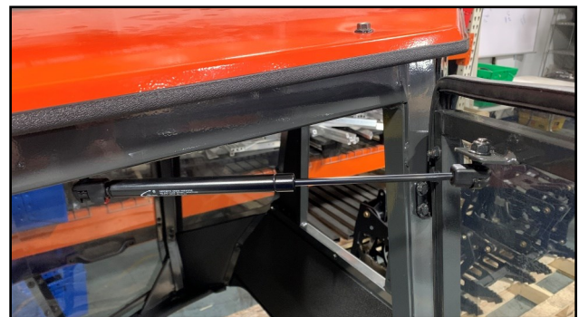
Fig. 11.1 (Attach Gas Shock)
