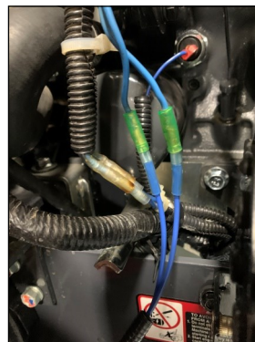
Fig. 7.12 (Connect Dynamo Wiring)
