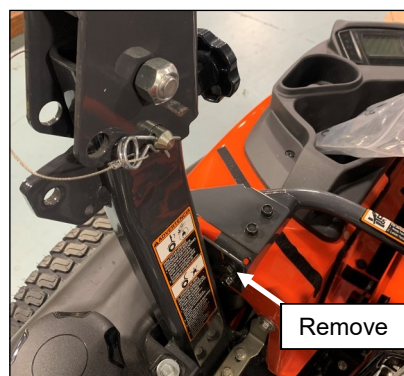
Fig. 3.3 (Remove upper bolt)
