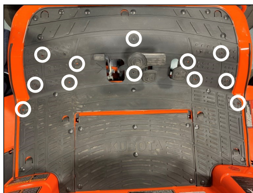
Fig. 4.3 (Remove Pine Tree Clips)
