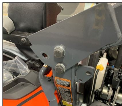
Fig. 3.6 (Tilt the ROPS)
