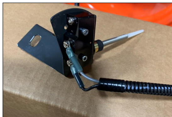
Fig. 7.5 (Connect Wires to Switch)
